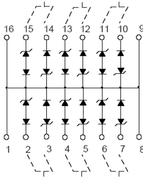
Note: Dash lines in schematic show intended pairing for bi-directional applications.
