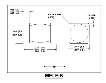
Note: The cathode side is marked with a dark colored band on one side of the diode body.
